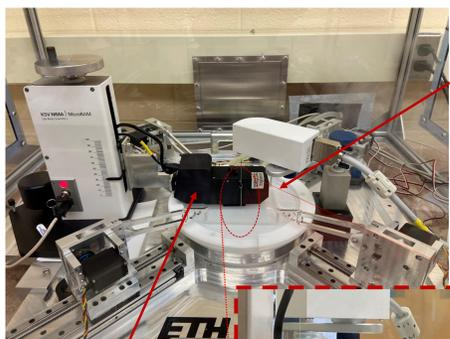
Elastic band is stretched around four step motors to allow precise interfacial deformation
