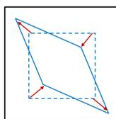
Quadrotrough has the ability to control the processing of the interface through pure shear and pure dilation/compression for better approximation of interfacial rheological parameters
