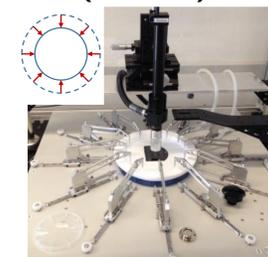
Instrumentation is created for pure dilation/compression, but unable to 'pre-shear' interface and investigate interfacial structure
