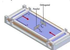
Interfacial viscoelastic moduli ( $K$ ,  $G$ ) convoluted with static compressibility  $\Pi_{\alpha\beta}(\Gamma)$ , creates orientation dependence of interfacial tension probe. As a result, there difficulty in determining parameters due to coupled shear and dilatational flows.
